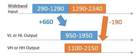
Important : DC must be provided on VL to power the 9646 and the wideband LNB (DC power pass from VL to V).
